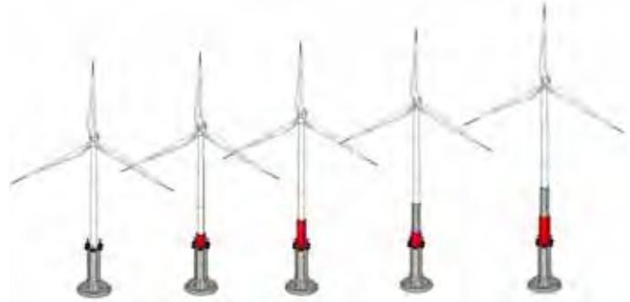
Figure 27: Tower lifting process
