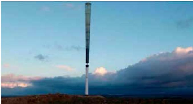
Figure 7: Bladeless Vortex Wind Turbines<sup>11</sup>
