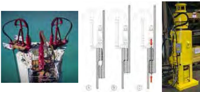
Figure 24, 25 and 26: Stand- jack positioning
