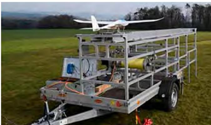
Figure 3: Linear Take-off System Tested by ABB Corporate Research<sup>6</sup>
